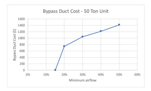
For limited VAV turndown, there is significant energy savings for fan systems that can turndown below the current 50% requirement.
